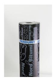
Pre-fabricated waterproofing membrane made of distilled bitumen and elastomeric polymers SBS and CPB (blend of copolymer polyolefin's) from metallocene catalysis polymerization, reinforced with a woven non woven single strand composite polyester, which gives the membrane high mechanical characteristics and excellent dimensional stability.
